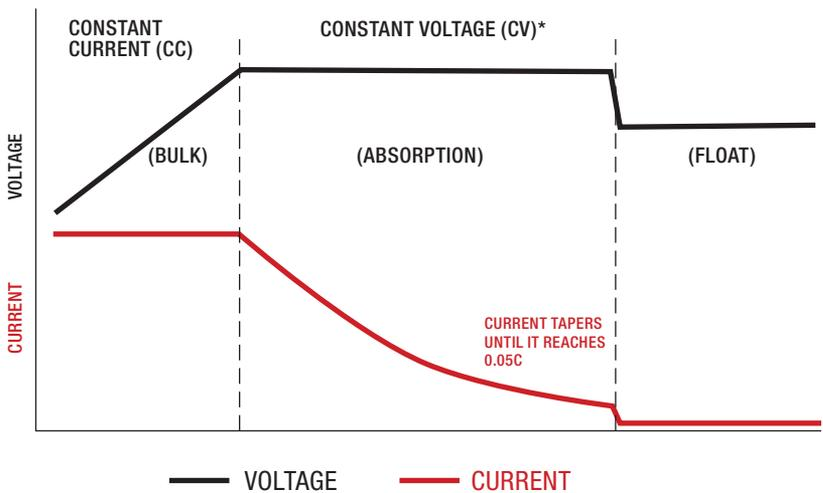
Representation of recommended 2-Stage Constant Current/Constant Voltage (CC/CV) charging. The dotted line represents the transition from CC to CV when the voltage limit is reached. Once the battery reaches the constant voltage limit, the battery is held by the charger at this voltage until the current decreases to 0.05C. At this point the battery is at 100% state-of-charge (SOC). Any current continuing to flow in the float stage is attributable to balancing activity of the BMS.
