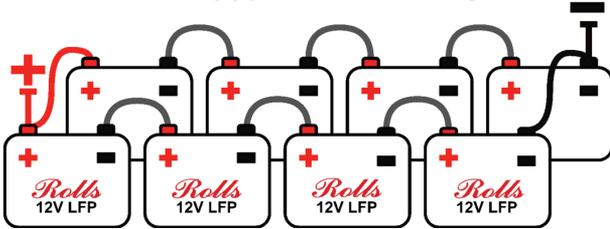
**NOTE:** Strings are independent. External connections should be staggered, i.e., the positive lead is connected to string one, whereas the negative lead is connected to string two.
