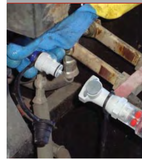
One connection waters all cells simultaneously
